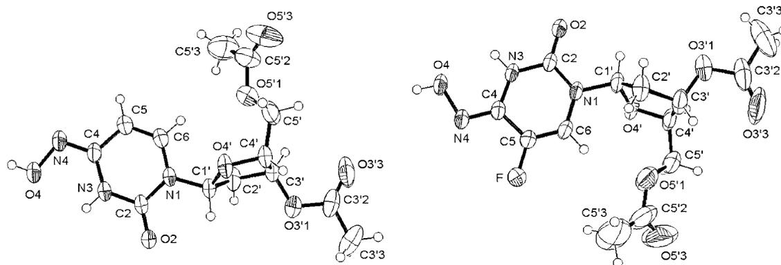
**Fig. 1.** ORTEP diagram at the 50% probability level and atom numbering for 3',5'-di-*O*-Ac-*N*(4)-OH-dCyd (left) and 3',5'-di-*O*-Ac-*N*(4)-OH-FdCyd. One of the five symmetry-independent molecules of 3',5'-di-*O*-Ac-*N*(4)-OH-dCyd is shown.
